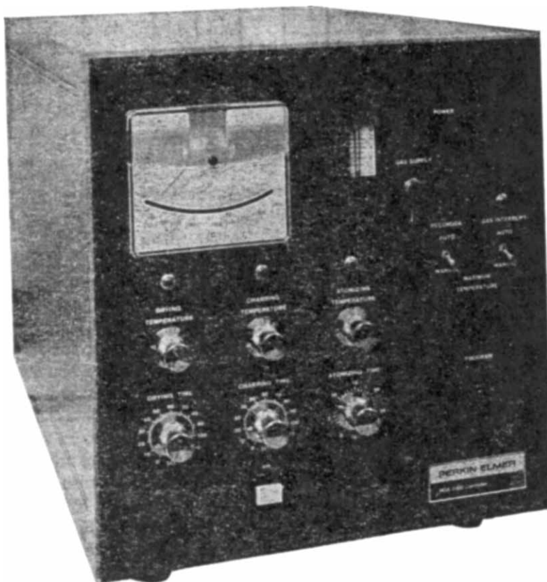
FIGURE 3 Control system for Perkin-Elmer HGA-2000 Graphite Furnace.
